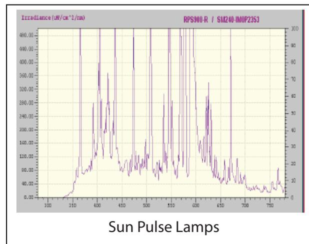
The spectral graphs above show three HPS lamps (left) and three Sun Pulse lamps (right) in a 30"x30"x26.75" Hood w/ glass at a 30" Distance
